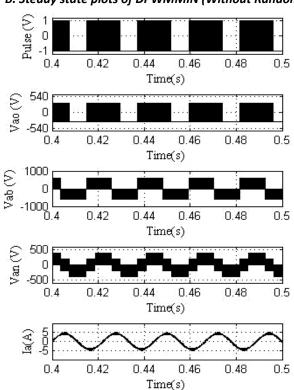
Fig.9 Pulses, Pole voltage, Line voltage, Phase voltage and stator current.
