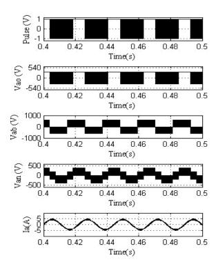
Fig12. Pulses, Pole voltage, Line voltage, Phase voltage and stator current.
