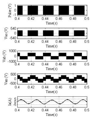
Fig.18 Pulses, Pole voltage, Line voltage, Phase voltage and stator current.
