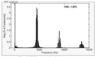
Fig.10 THD analysis of stator current
