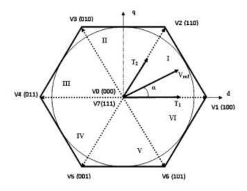
Fig.1: Voltage space vectors for SVPWM
