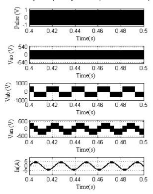
Fig.6 Pulses, Pole voltage, Line voltage, Phase voltage and stator current.
