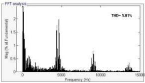
Fig.19 THD analysis of stator current
