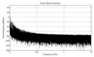
Fig.17 Acoustic noise for VDR SVPWM
