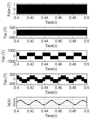
Fig. 15 Pulses, Pole voltage, Line voltage, Phase voltage and stator current.
