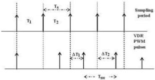
Fig 2. Timing diagram for VD-RPWM implementation.
