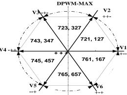
Fig.4: Voltage space vectors for DPWMMAX
