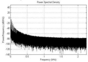
Fig. 20 Acoustic noise for VDR DPWMMIN
