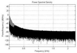
Fig. 23 Acoustic noise for VDR DPWMMAX
