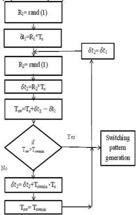
Fig 3 Flow chart of a VDPWM algorithm
