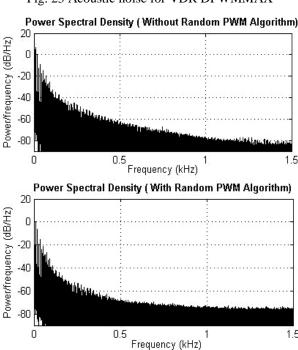
Fig. 24 Acoustic noise Comparision without and with random PWM Algorithm
